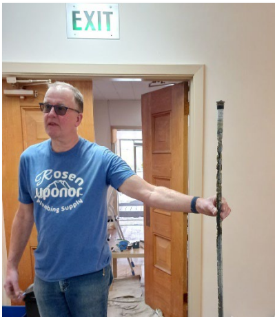
Dean Paulsen showing the old water heater anode rod he replaced so the church had hot water again!
